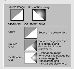
You can achieve interesting effects with compositing when the initial images are drawn with partially transparent paint. (Transparency is specified by *coverage*, a indicator of paint opacity.) In a typical compositing operation, paint that's partially transparent won't completely cover the image it's placed on top of; some of the other image will show through. The more transparent the paint is, the more of the other image you'll see.
