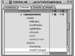
Outlets and actions already defined by the superclass (or by its superclasses) appear in gray text. Add the outlets and actions shown in black text.
